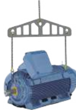
Figure 7 - Lifting with vertical chains.
