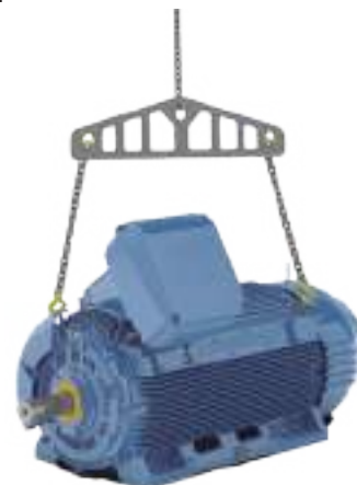
Figure 8 - Lifting with inclined chains.
